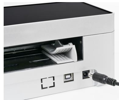
2.2 Plug the power cord into the power adapter. Plug the power adapter into the power interface on the back of the printer. Plug the other end of the power cord into a power outlet.
