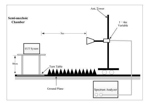
The radiated emission tests were performed at the 3 meters distance, using the setup accordance with the ANSI C63.4-2014. The specification used was the FCC Part 15B Class B limits.
