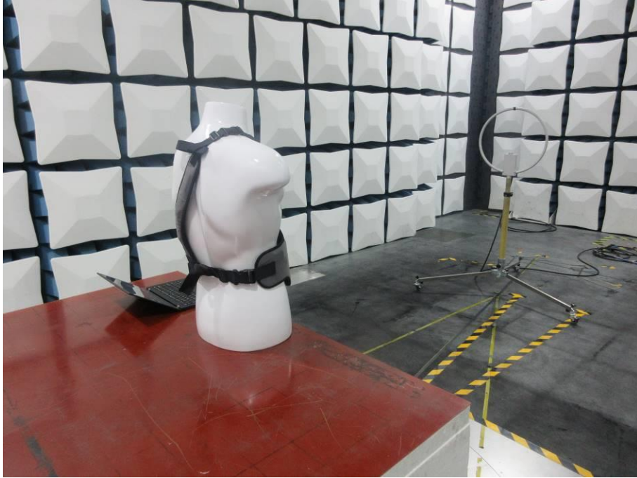
RADIATED RF MEASUREMENT SETUP (9KHz ~ 30 MHz)
