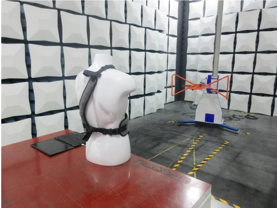
RADIATED RF MEASUREMENT SETUP (30MHz ~ 1 GHz)
