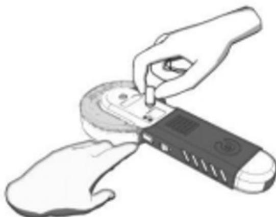
**Figure 7-2: Schematic Diagram of turning-on the Capsule**
