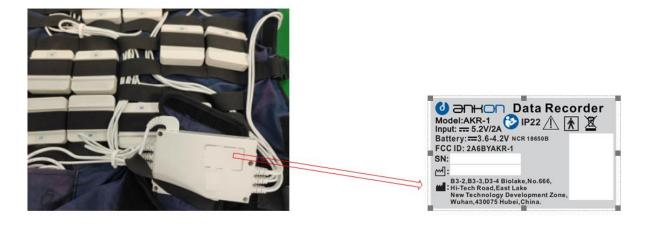
PS: Label locates on the bottom of the device
