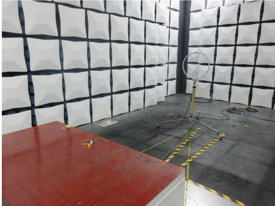
RADIATED RF MEASUREMENT SETUP (9KHz ~ 30 MHz)
