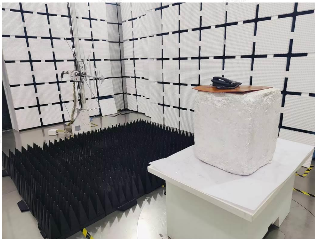
Radiated Emissions Measurement (Below 1GHz)
