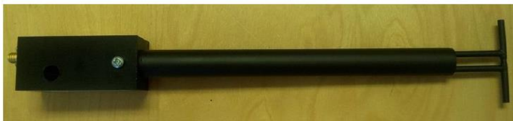
Figure 1 – MVG COMOSAR Validation Dipole
