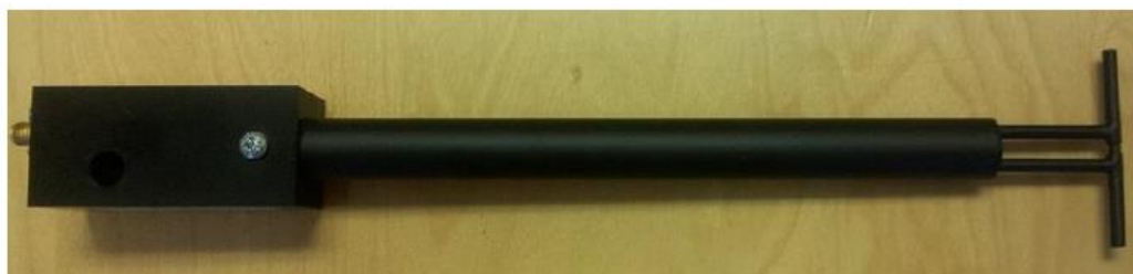
Figure 1 – MVG COMOSAR Validation Dipole
