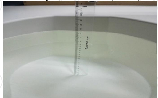
The Body Liquid of 2450MHz (15.3cm)
