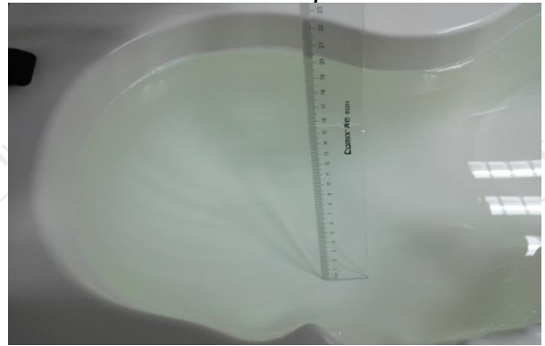
The Head Liquid of 2450MHz (15.6cm)
