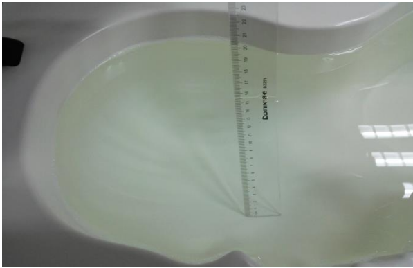
The Head Liquid of 1900MHz (15.5cm)
