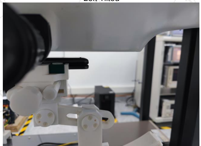
Body worn – Back close (10mm)
