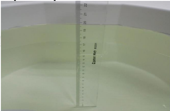
The Body Liquid of 835MHz (15.4cm)
