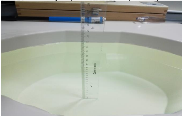
The Body Liquid of 1900MHz (16.4 cm)
