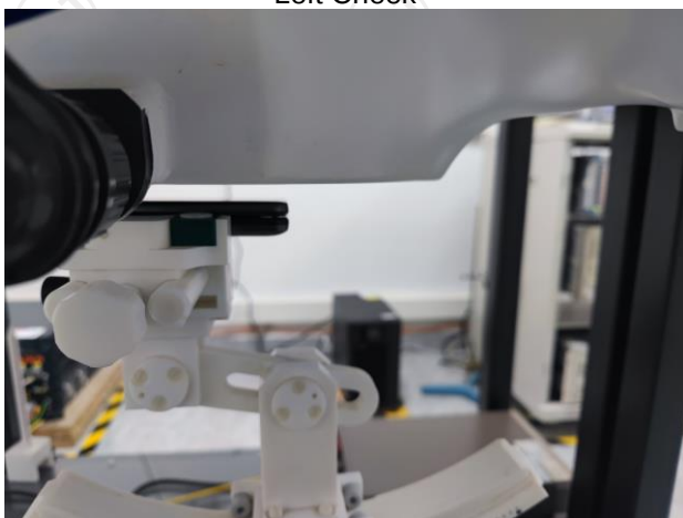
Body worn – Front close (10mm)
