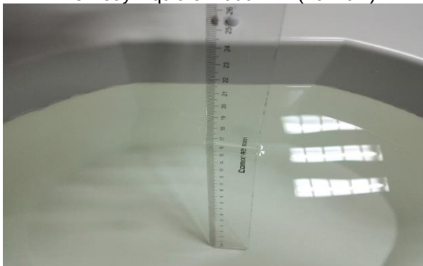
The Body Liquid of 2600MHz (16.5cm)
