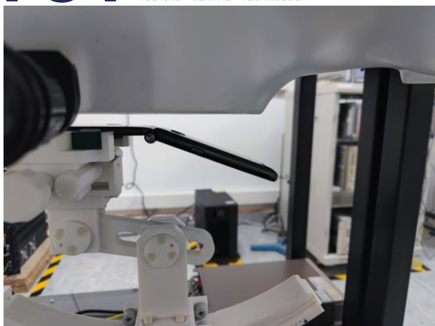
Body worn – Front open (10mm)
