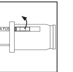
5. Close fuse cover. Slide closed the fuse access cover on top of attachment plug.
