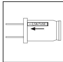
2. Open fuse cover. Slide open fuse access cover on top of attachment plug towards blades.
