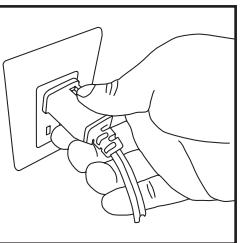
1. Grasp plug and remove from the receptacle or other outlet device. Do not unplug by pulling on cord.
