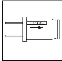
3. Remove fuse carefully. Push the fuse from the other side or turn fuse holder over to remove fuse.
