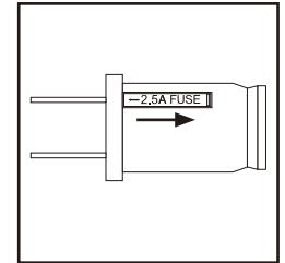
5. Close fuse cover. Slide closed the fuse access cover on top of attachment plug.
