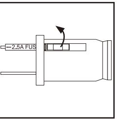
3. Remove fuse carefully. Push the fuse from the other side or turn fuse holder over to remove fuse.
