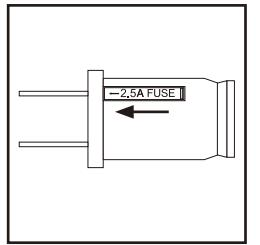
2. Open fuse cover. Slide open fuse access cover on top of attachment plug towards blades.
