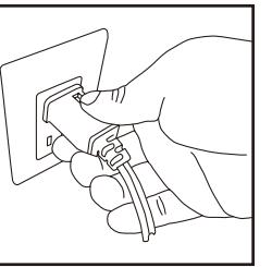
1. Grasp plug and remove from the receptacle or other outlet device. Do not unplug by pulling on cord.
