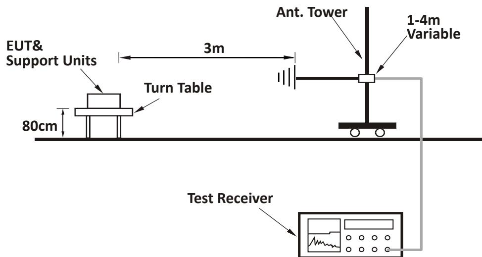
**TEST REPORT****For Radiated emission above 1GHz:**
