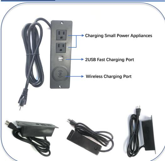
System Specifications / Model: YY134-08Input: 100-240Vac / 50/60hz / 12A MaxOutput: usb1 / 5V 2.4A ; usb2 / 5V 2.4Ausb1 & usb2 / 5V 2.4AWireless Charging 10W MaxAC Socket: 1500W maxReceiving Distance: 2-6mmConversion Efficiency: ≥ 75%Operating frequency: power port / 20k-50k Hzwireless charging / 115k-205k Hz
