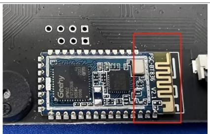
The antenna is PCB antenna. The best case gain of the antenna is 2dBi.
