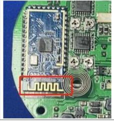
The antenna is PCB antenna. The best case gain of the antenna is 2dBi.
