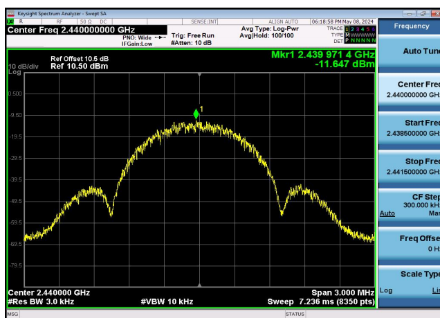
Power spectral density: 2440MHz
