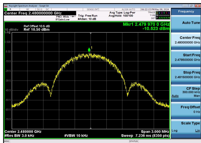
Power spectral density: 2480MHz
