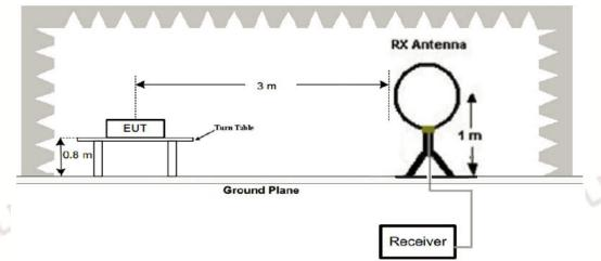
2. Radiated Emission Test-Up Frequency 30MHz~1GHz
