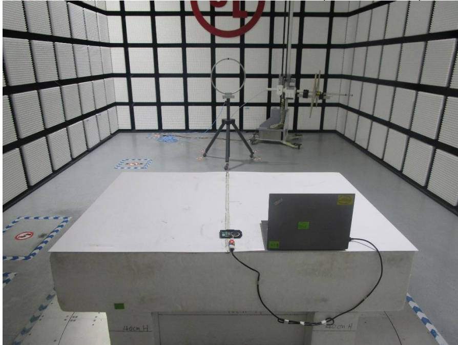
RADIATED RF MEASUREMENT SETUP (Below 30MHz)
