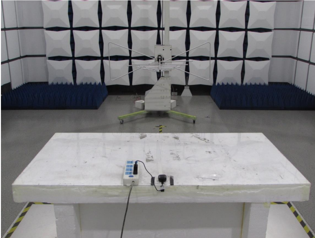
Radiated Emission Above 1GHz
