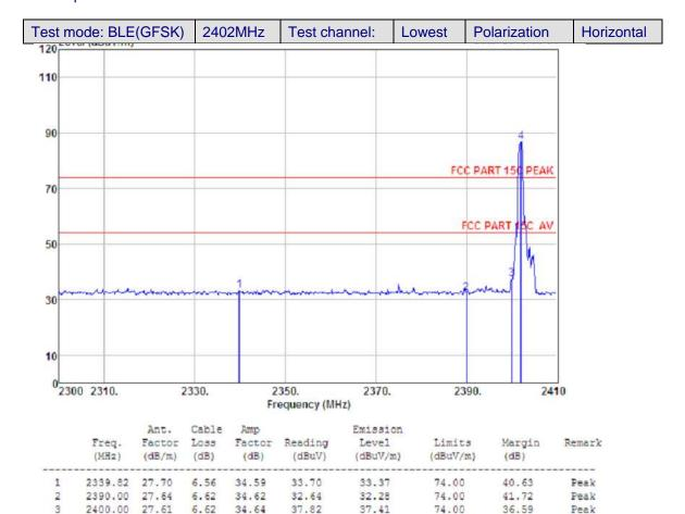
Remarks: 1. Emission Level= Antenna Factor + Cable Loss - Amp Factor + Reading.
