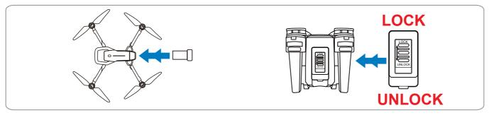
⚠ ① Insert the battery into the rear of the drone in the right direction (the tab on the battery should be facing up)
