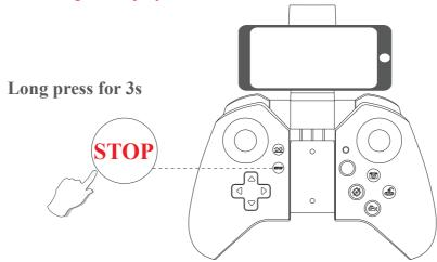
As shown above, long press the Emergency Stop button for 3 seconds, the motor will stop immediately.
