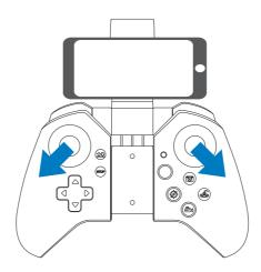
Move the Left Control Stick to lower left in 45° and the Right Control Stick to lower right in 45° at the same time, the indicator light on drone will blink and turn solid that indicates the calibration is completed.
