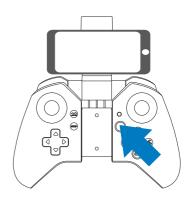
④ Push the throttle joystick up then down to pair the drone with the transmitter. The indicator light on the drone will turn solid if the drone is paired successfully.
