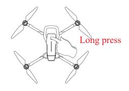
② Place the drone on a flat and level surface with the head forward and the tail facing towards the pilot.
