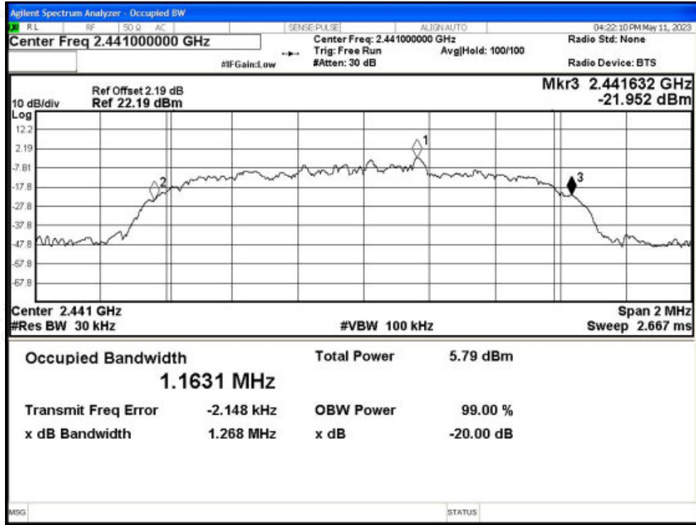
-20dB Bandwidth NVNT 2-DH5 2480MHz Ant1
