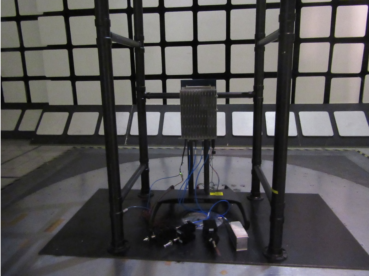
Figure 2 – Radiated Emissions Setup – Photo 2
