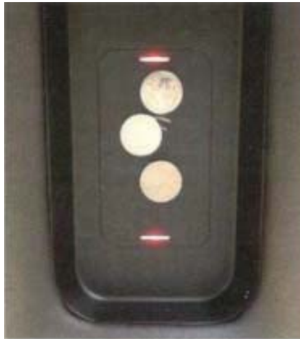
FOD Protection Feature - Red LED Indicator Lights
