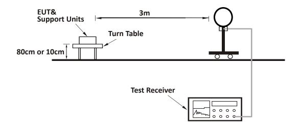
For Radiated emission 30MHz to 1GHz:
