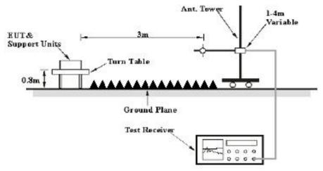
The radiated emissions were performed in the 3 meters distance, using the setup accordance with the ANSI C63.10-2013. The specification used was the FCC 15.205, 15.209, and FCC 15.231 limits.
