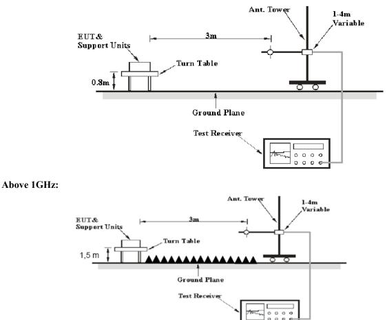
The radiated emissions were performed in the 3 meters distance, using the setup accordance with the ANSI C63.10-2013. The specification used was the FCC 15.205, 15.209, and FCC 15.231 limits.
