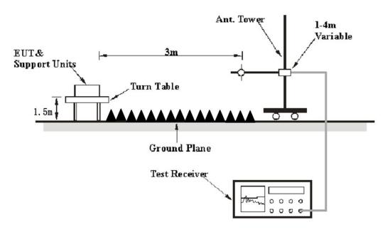
The radiated emission tests were performed in the 3 meters test site, using the setup accordance with the ANSI C63.10 - 2013. The specification used was the FCC 15 § 15.209, 15.205 and 15.231.
