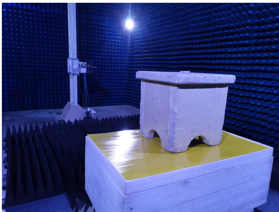
Photo of Radiated Emission Measurement (Above 1GHz)
