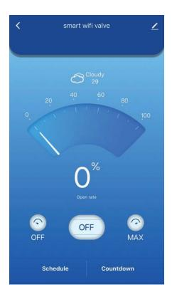
12. Tap "OFF" on the left side. The valve will close completely.
