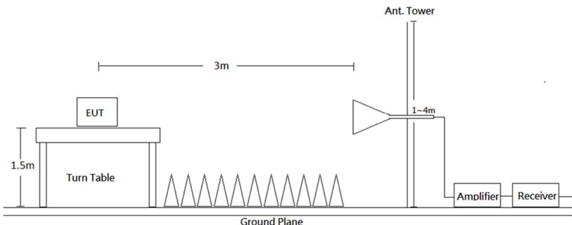
Radiated emission tests were performed in the 3 meters chamber test site, using the setup accordance with the ANSI C63.10-2020. The specification used was the FCC Part 15.209 and FCC 15.407 Limits.
