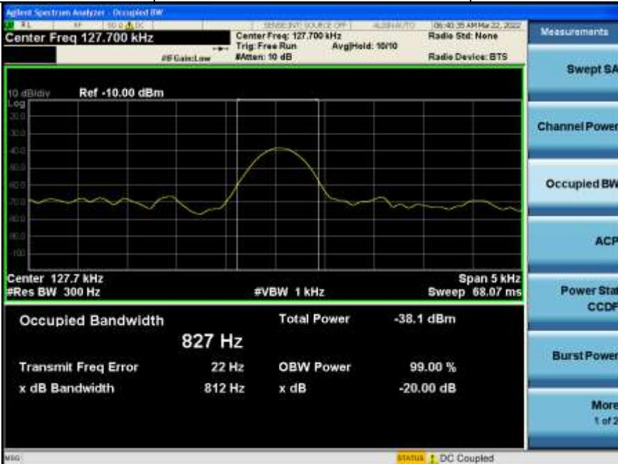
The screenshot shows the Agilent Spectrum Analyzer interface. The main display is a log scale plot with a single prominent peak at 127.7 kHz. The measurement table on the right provides the following data:
