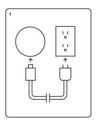
1 Connect the cable to the charging pad and plug in to an electrical outlet.
