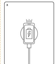
**3** Check the light on the sides of the charging pad to ensure that it is charging properly.
