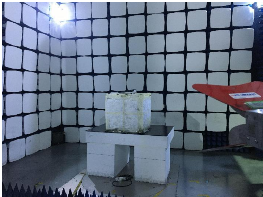
Radiation Emission Test Setup (1GHz to 18GHz)
