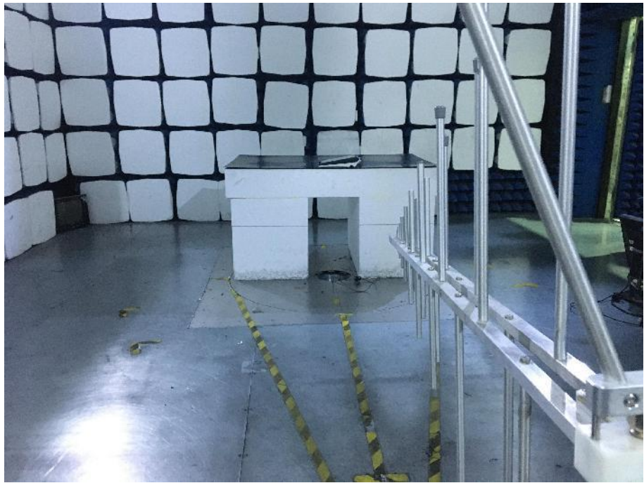
Radiation Emission Test Setup (30MHz to 1GHz)
