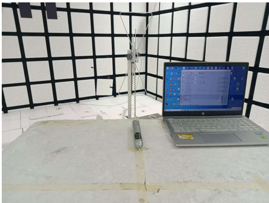
Radiated spurious emission Test Setup-1(Below 1GHz)
