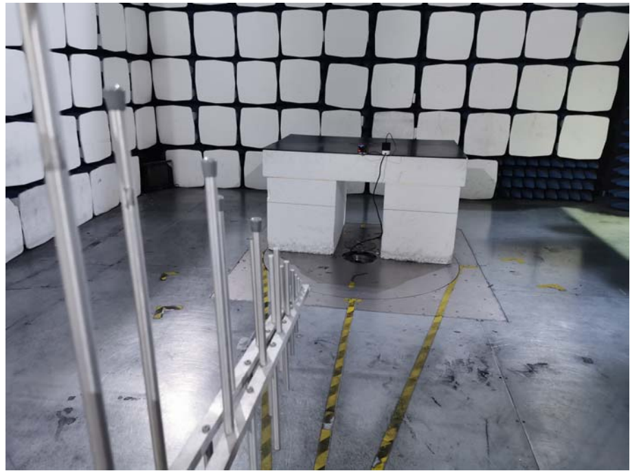
Radiation Emission Test Setup (30MHz to 1GHz)
