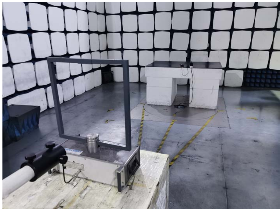
Radiation Emission Test Setup (Below 30MHz)
