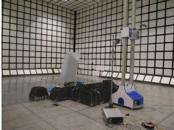
Radio-frequency radiated emissions 26 GHz to 40 GHz
