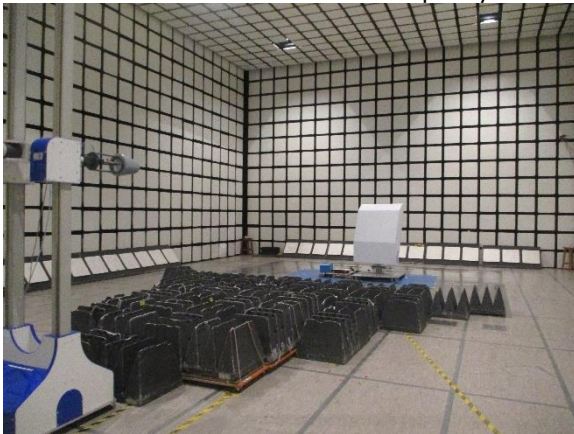
Radio-frequency radiated emissions 1 GHz to 18 GHz
