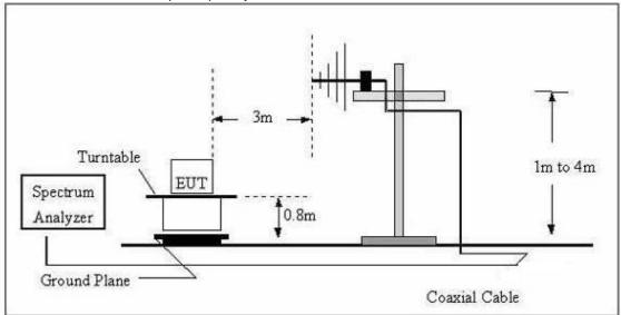
(C) Radiated Emission Test-Up Frequency Above 1GHz
