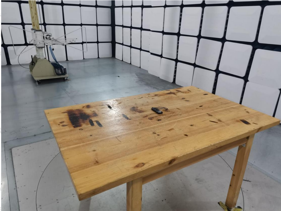
Photo of Radiation Emission Test
