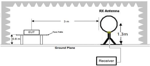
Radiated Emission Test Set-Up, Frequency below 1000MHz
