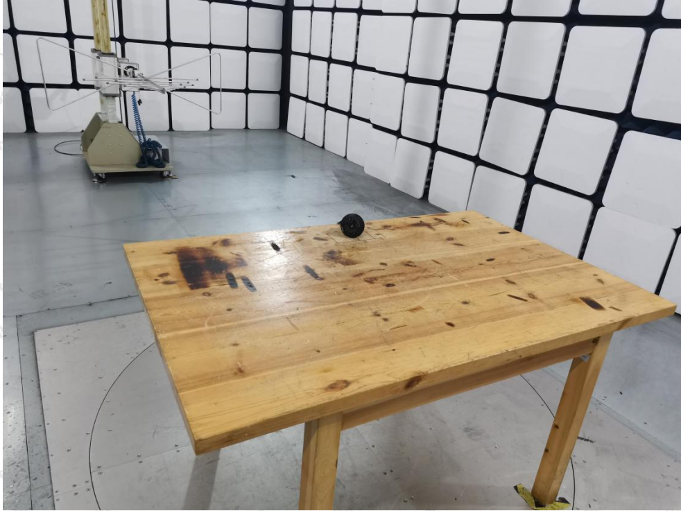
Photo of Radiation Emission Test
