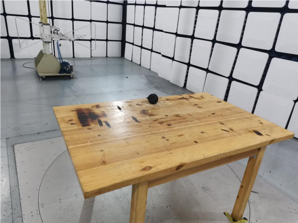
Photo of Radiation Emission Test
