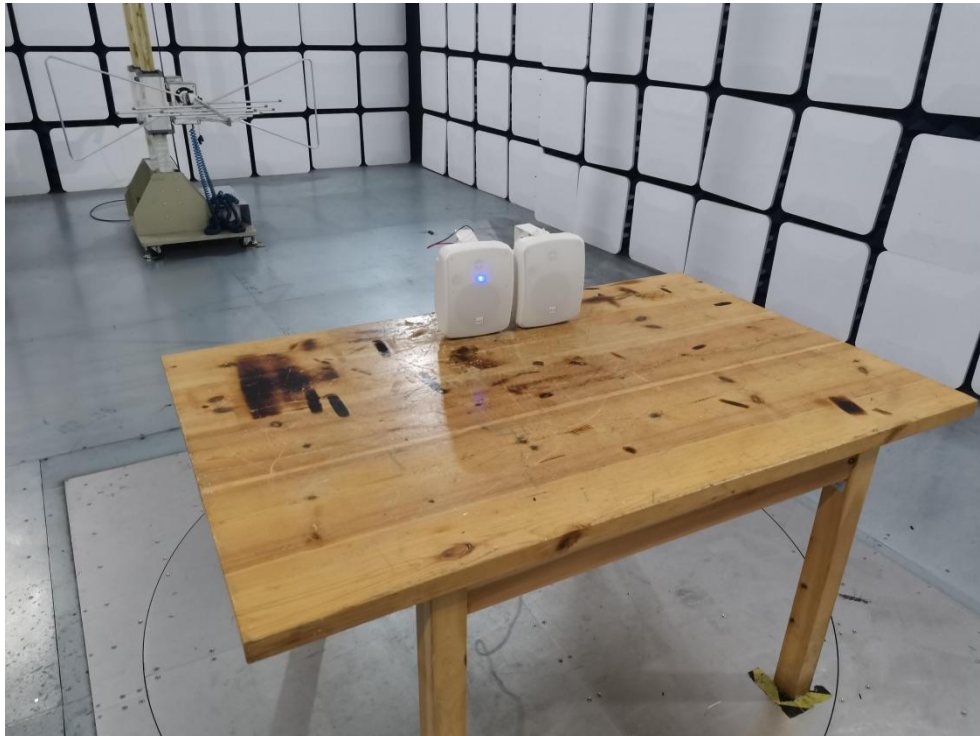
Photo of Radiation Emission Test
