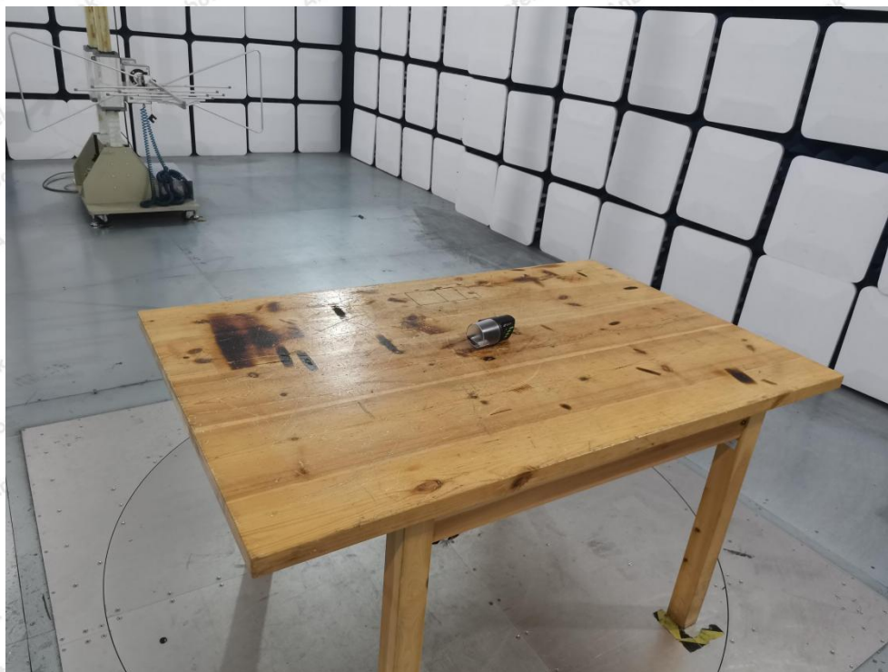
Photo of Radiation Emission Test
