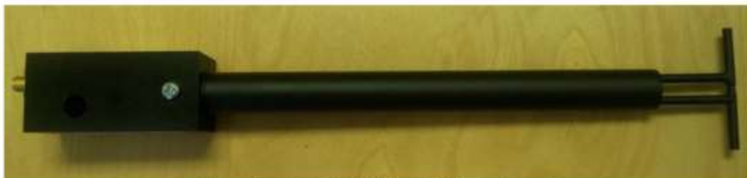
Figure 1 – MVG COMOSAR Validation Dipole
