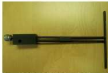
Figure 1 – MVG COMOSAR Validation Dipole
