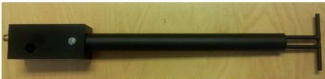
Figure 1 – MVG COMOSAR Validation Dipole
