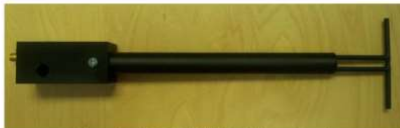
Figure 1 – MVG COMOSAR Validation Dipole
