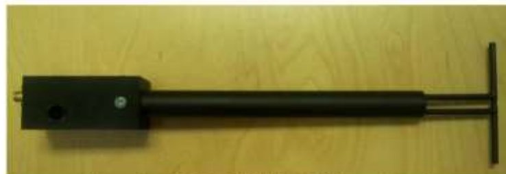
Figure 1 – MVG COMOSAR Validation Dipole
