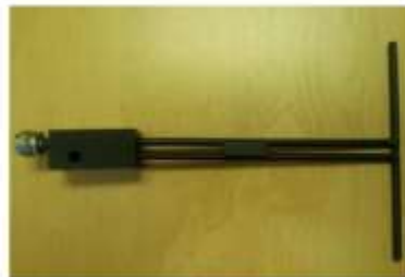
Figure 1 – MVG COMOSAR Validation Dipole
