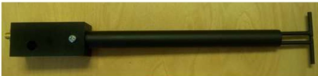
Figure 1 – MVG COMOSAR Validation Dipole
