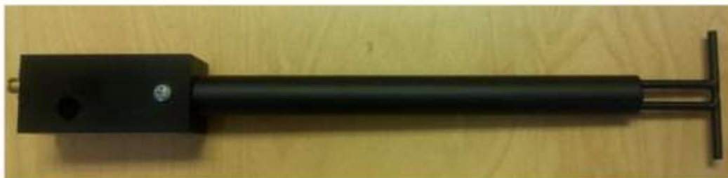
Figure 1 – MVG COMOSAR Validation Dipole
