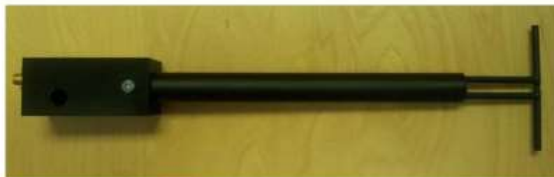
Figure 1 – MVG COMOSAR Validation Dipole
