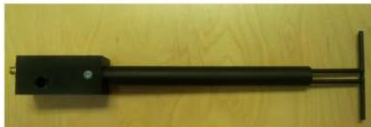
Figure 1 – MVG COMOSAR Validation Dipole
