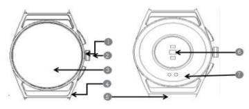
①power key ②function key ③TFT monitor ④strap card ⑤wristband ⑥sensor ⑦charging port
