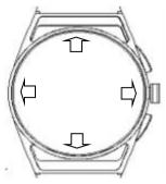
Slide: Call out the control center Slide up: Call out the notification center lide right: call out function menu Left slide: call out quick function Long press: call out the dial switch
