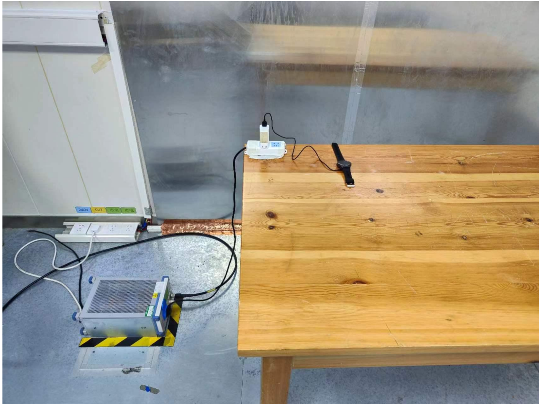
Conducted emission test setup
