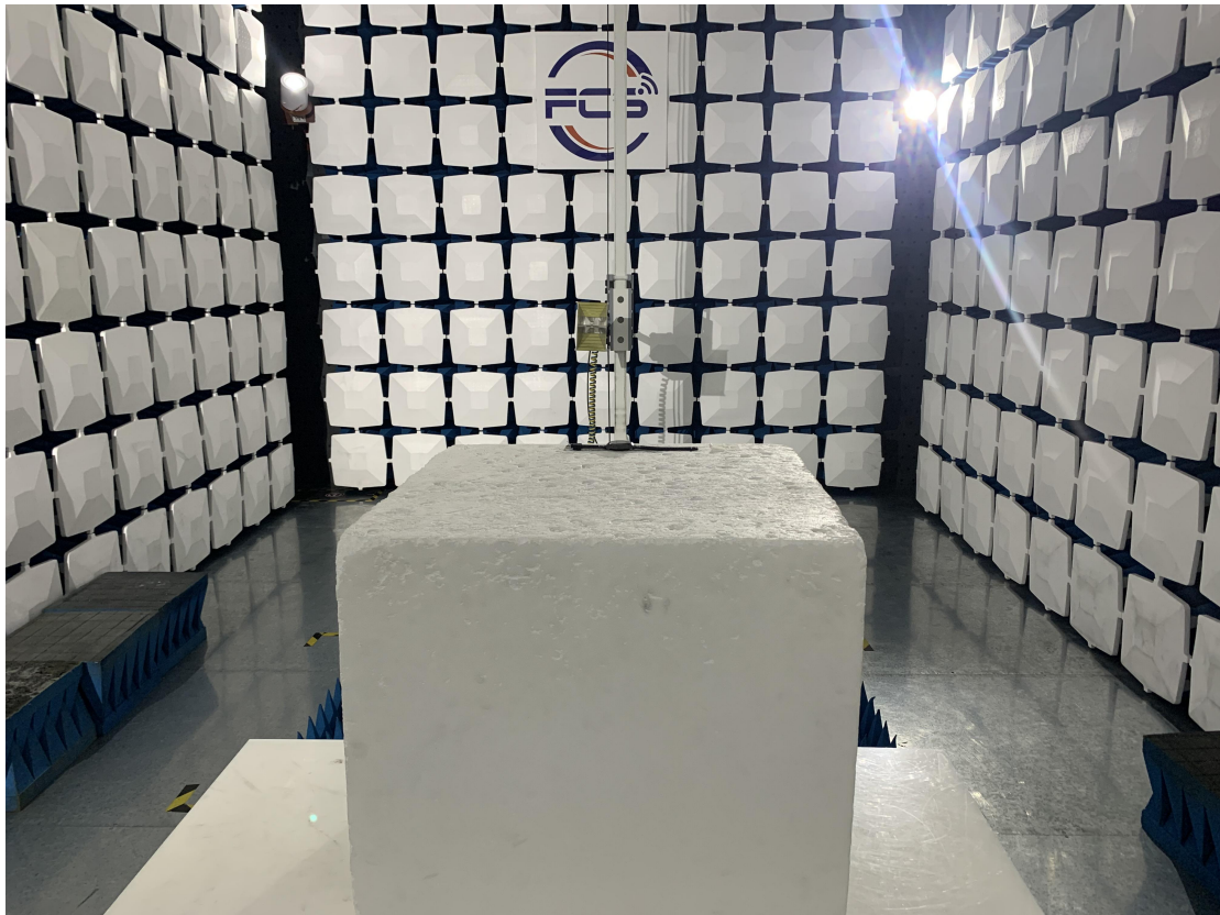
Above 1GHz for radiated emission test setup
