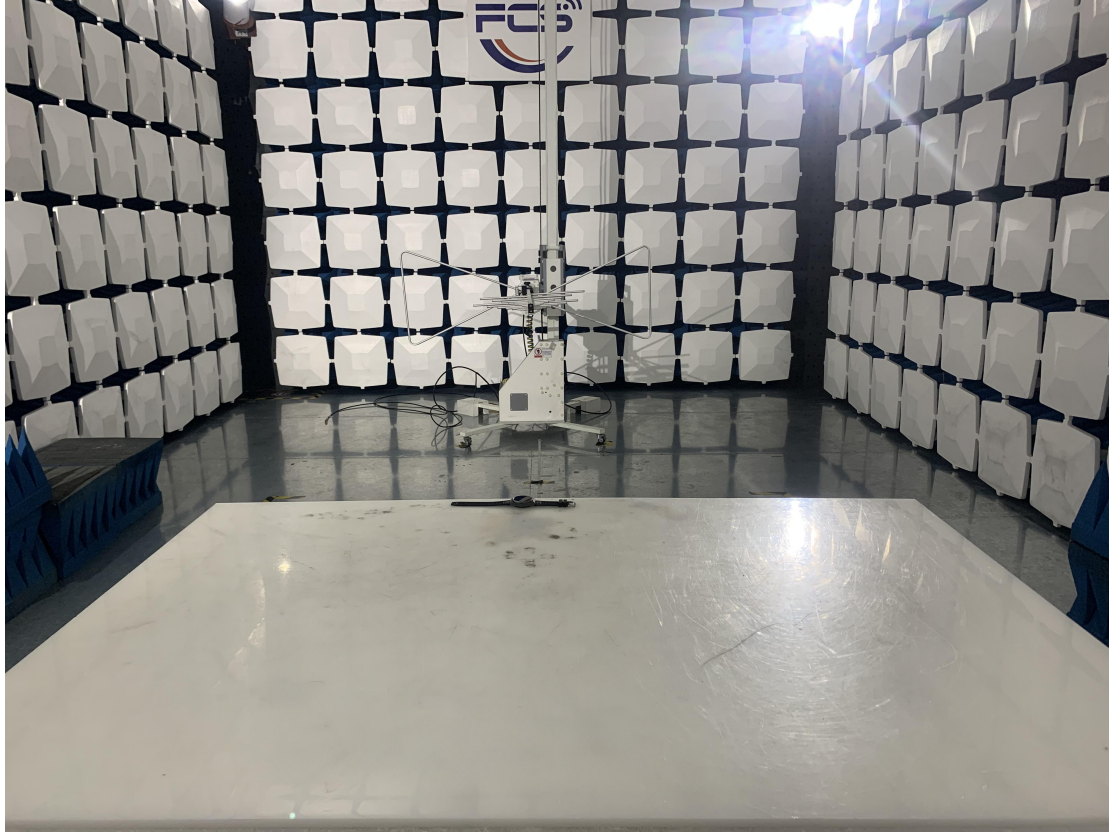
Below 1GHz for radiated emission test setup
