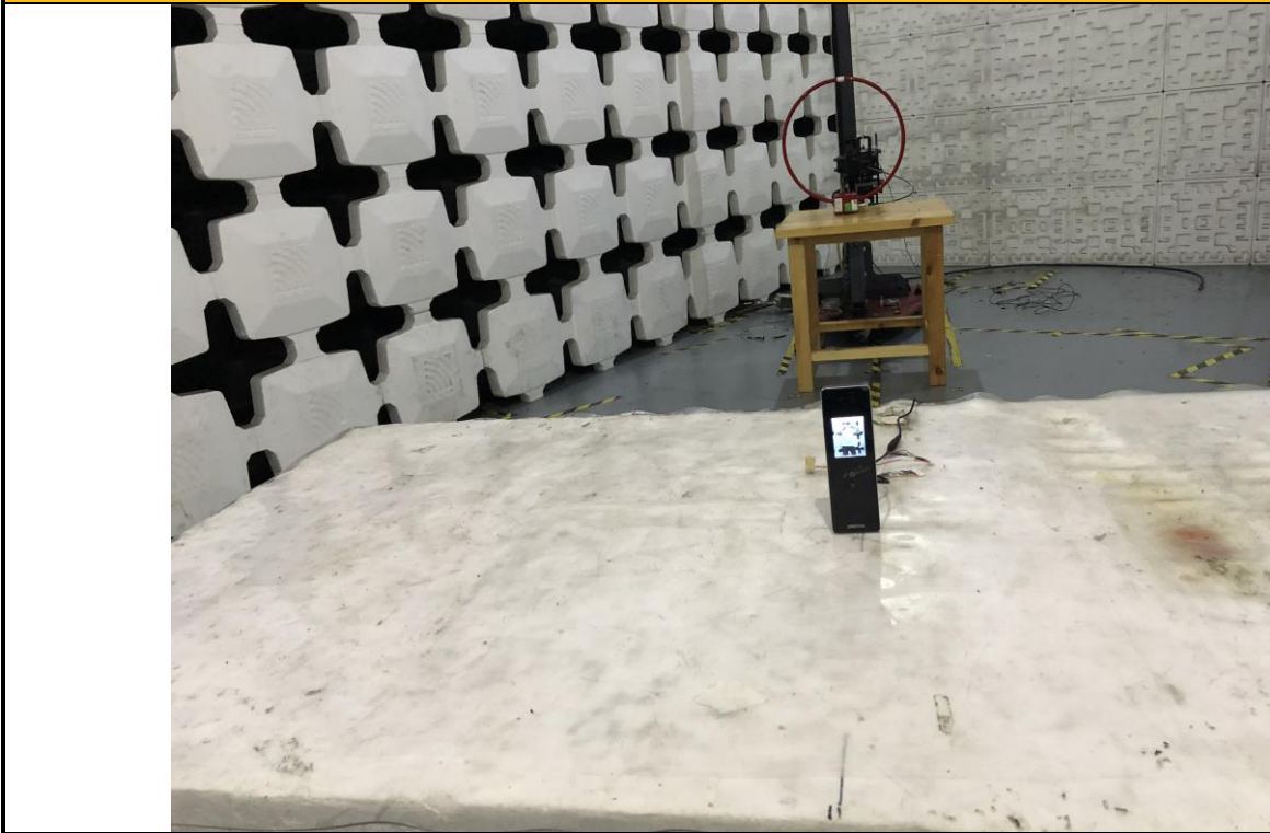
Radiated emission Test Setup (Below 30MHz)
