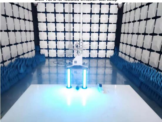
Blow 1GHz for radiated emission test setup
